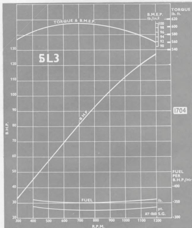
These graphs are made from figures regularly observed during the ordinary tests of the engines ; they are in no sense mere laboratory results. Large scale prints of the graphs are available on application.
