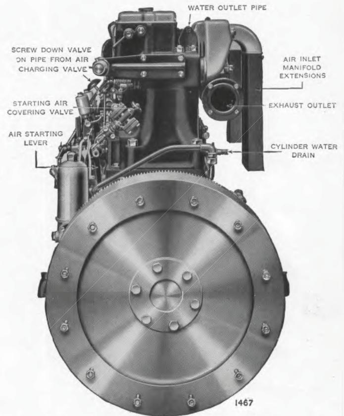
**Fig. 14** FLYWHEEL-END VIEW OF RAIL-TRACTION ENGINE
