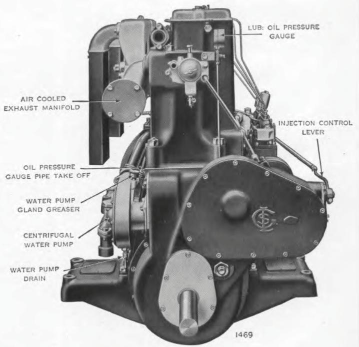
**Fig. 16** FORWARD END VIEW OF A RAIL TRACTION TYPE ENGINE
