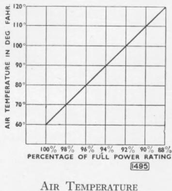
**Example.**—Given that the engine has to work at an altitude of 3,000 feet above sea level with an air temperature of 90° F. From the diagrams, we read the following coefficients of reduction :—
